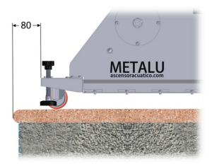
3. Place the **safety bar vertically**, such that it <u>rests in the hinge space</u> so that it actuates the micro-switch of the electrical system. The back supports shall end up below the level of the back wheels, leaving them suspended in the air.
